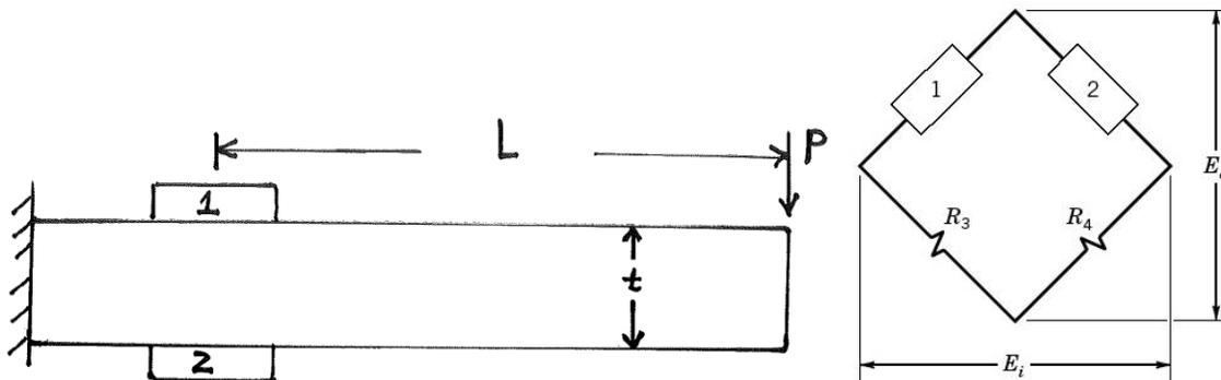
**Figure 2.** Strain gages mounted on a cantilever beam with end closer to strain gages clamped and strain gages connected to the arms 1 and 2 of the Wheatstone bridge circuit shown on the right.
