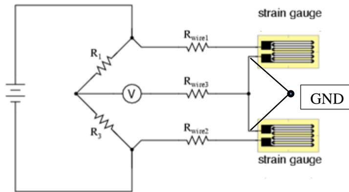
**Figure 1.** Electrical schematic of Wheatstone bridge circuit with strain gages attached to arms 3 and 4 of the bridge circuit. (From How sensors work: strain gage web site: <http://www.sensorland.com/HowPage002.html>).
