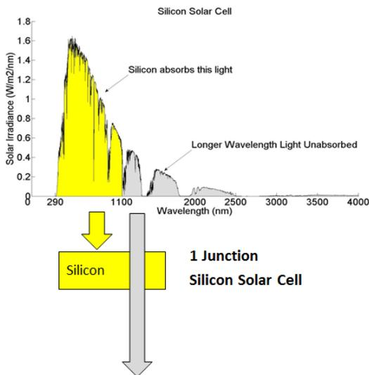
Figure 1: Single junction solar cell. Source: [14]
