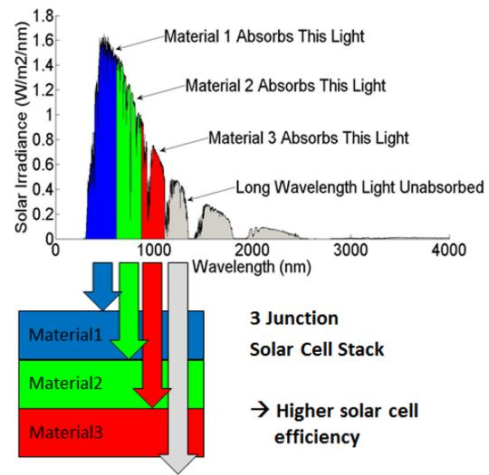
Figure 2: Multi-junction solar cell. Source: [14] cells.
