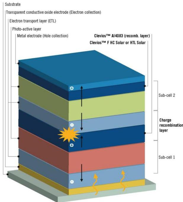
**Figure 3: Tandem solar cell. Source: [16]**
