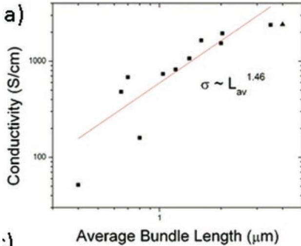
Figure 4: Conductivity vs Avg. bundle length. Source: [4]
