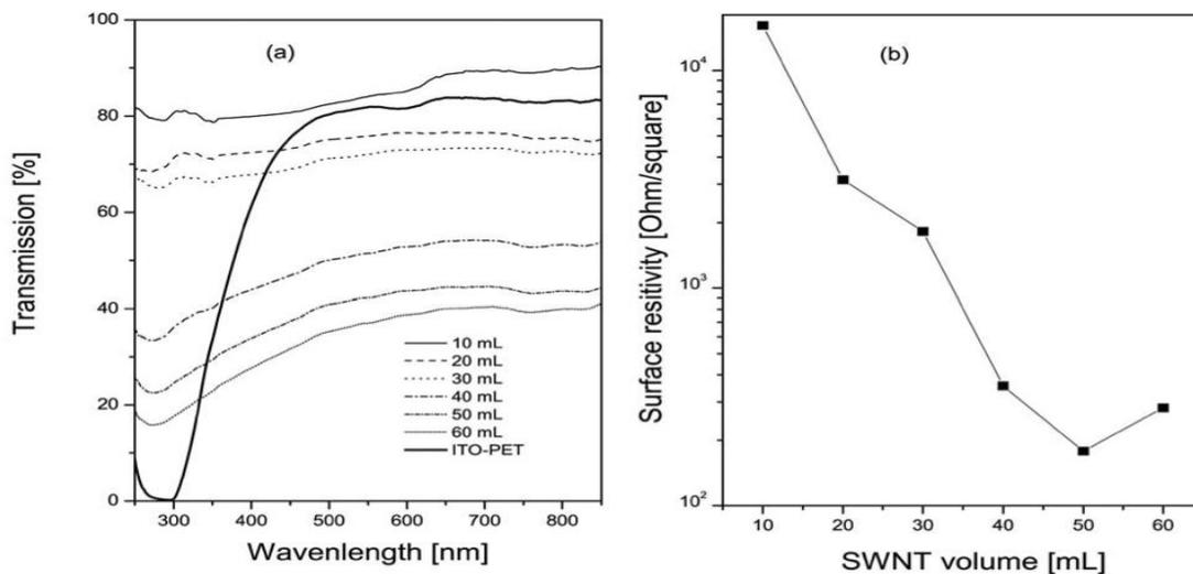
Figure 5: Transmission and resistivity for CNT films. Source: [6]
